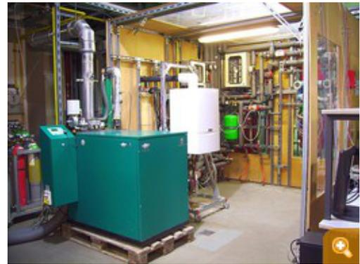
Micro-CHP system on the test rig
